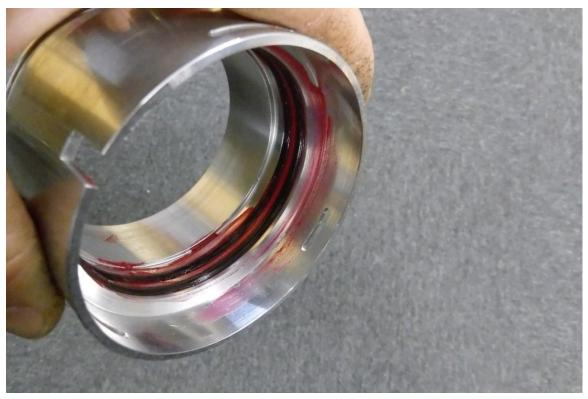
8. Fit the coupler to the intercooler. It is a very tight fit so you may want to use a rubber mallet to tap it into place. Make sure the retaining clip is attached once in place, as this will keep the coupler securely in position.
