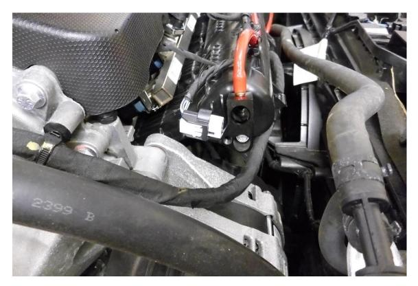
14. Using a 5mm Allen key secure the map sensor to the vacuum tap with the supplied M6 fastener and washer. Re attach the wiring loom to the sensor.
