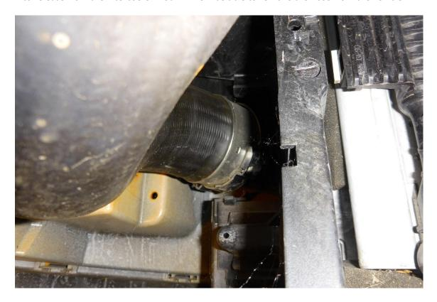
7. Using a flat blade screwdriver remove the retaining clip from the OE boost pipe. Take the coupler from the FMDV35 kit and lubricate the O-rings as this will make fitment easier.
