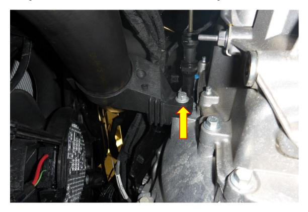
6. Using a flat blade screwdriver, lever the retaining clip upwards to allow the coupler on the hose to release from the intercooler. You will now be able to remove the hose from the vehicle.
