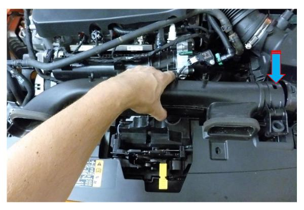
3. Using a 7mm socket and ratchet or flat blade screwdriver loosen off the hose clamp securing the boost pipe to the throttle body.
