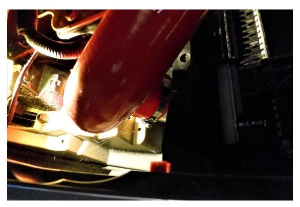
**10.** Using a 7mm socket and ratchet secure the other end of the silicone hose #2047 to the throttle body elbow with the supplied 40-60 hose clamp.
