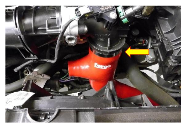
11. Take the Forge valve from the FMDV35 kit and attach the supplied 4mm vacuum hose to the vac port, secure it with a supplied cable tie. Using a 7mm socket and ratchet secure the valve to silicon hose #2047 using hose clamp 20-32. Run the vac hose as shown in the picture below and secure with supplied cable ties.
