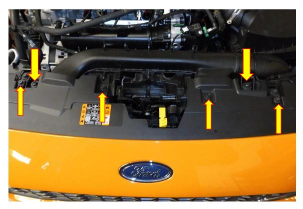
2. Push in both retaining tabs attaching the intake ducting to the airbox, this will then allow you to remove the intake ducting from the vehicle.
