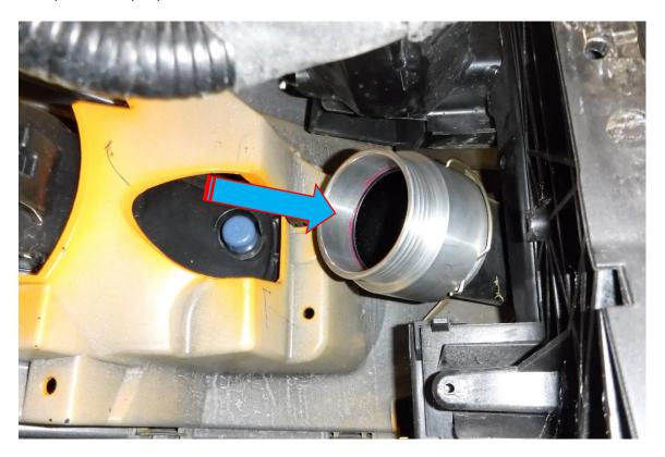
9. Using a 7mm socket or flat blade screwdriver secure large end of the of the silicone hose #2047 with the supplied 60-80 hose clamp.
