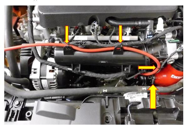
**12.** Unplug the wiring loom from the map sensor and using a 7mm socket and ratchet remove the fastener attaching the sensor to the inlet manifold. The sensor can now be removed.
