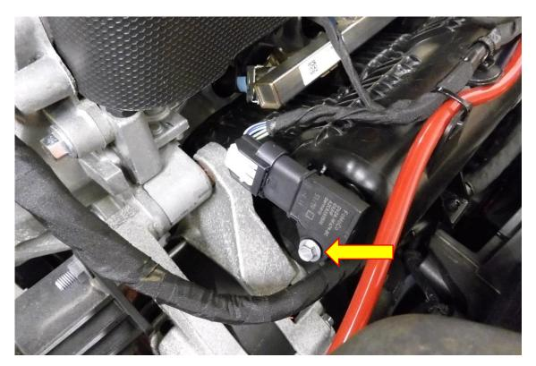
13. Using the original fastener secure the Forge machined vacuum tap to the inlet manifold. Using side cutters or a knife cut the 4mm vacuum hose to the correct length in order for it to fit the vacuum tap.
